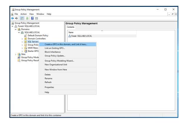
2. Within the GPO open, right click on the new GPO and select Edit and go to "Computer Configuration\Policies\Administrative Templates\Windows Components\Windows Remote Management (WinRM)\WinRM Service". Enable "Allow remote server management through WinRM" or "Allow automatic configuration of listeners" depending on your OS.
