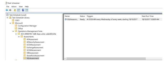
6. During collection and analysis, data is temporarily stored under the **WorkingDirectory** folder that was configured during setup, using the following structure:
